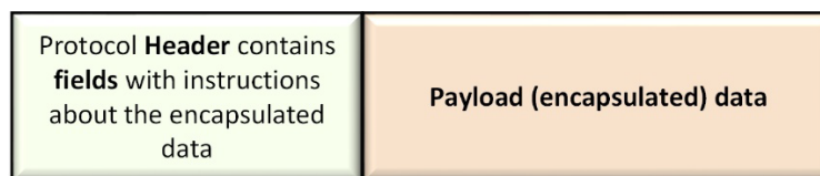
Protocol header and encapsulated data
